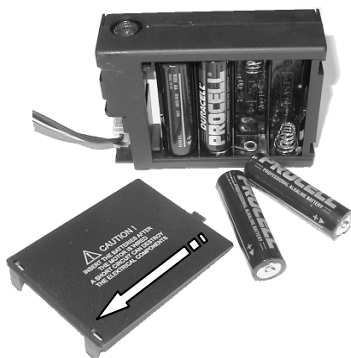
FIGURE 9 RECEIVER BATTERY REPLACEMENT
