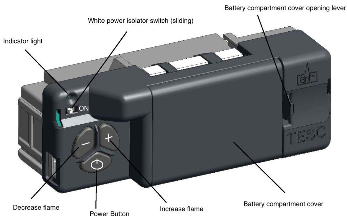
The power of the burner can be adjusted up and down by pressing the – and + buttons. After fitting the batteries and replacing the cover the fire can now operate. Slide the power isolator switch to the right to the on / I position.
