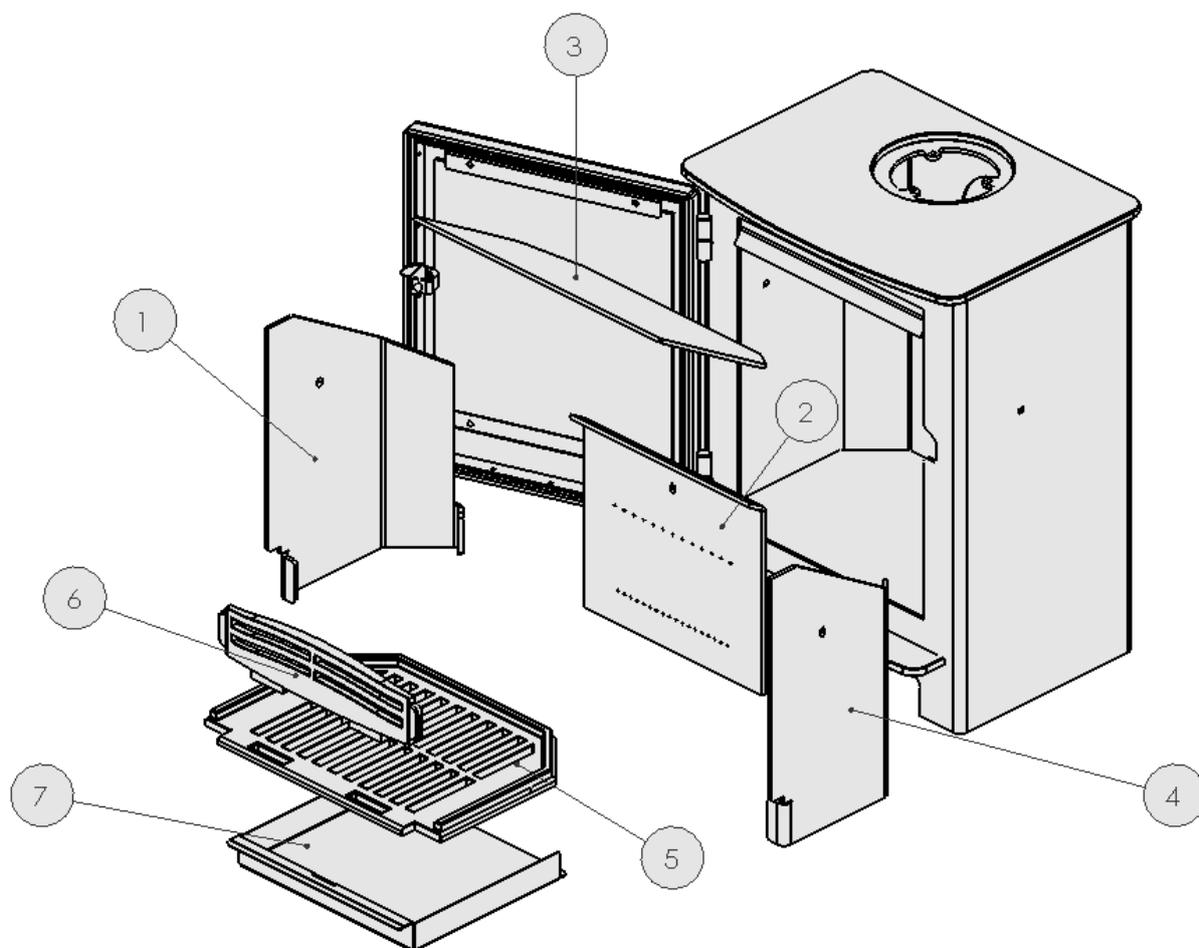
To refit the internals follow the numbered sequence from 1 – 7. The firebricks should be fitted with the fibre paper on the LHS, RHS and rear components, the fibre paper should be sandwiched between the fire brick and the main body, these are then held in position by the retaining screws, small gaps are acceptable between the firebricks. Be careful not to trap or squash fingers at this stage.
