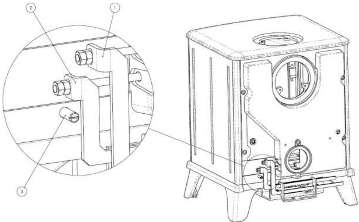
If the stove is being installed into a property which is not in a smoke control zone, you can simply screw the threaded rod into the stove (this will allow the slider to fully close and cut off the air supply)
